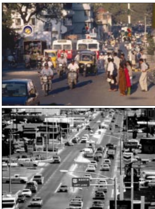
Fig 3 In many less motorised countries a disparate mix of road users share the same roads (top), so traffic engineering measures will be required that are different from those that have been successful in motorised countries, where traffic mixes are more homogeneous (bottom)
